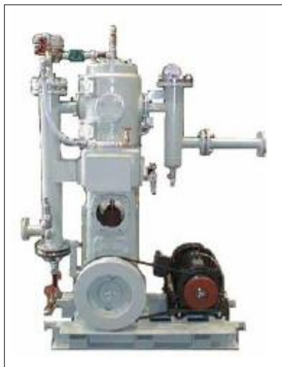
A gas compressor similar to this will be installed at the completed well and will operate daily.
